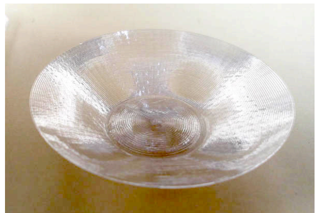
Figure 3. A small plate printed by the helical printing method
