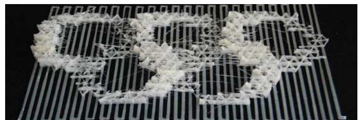
(b) Printed support (Thin strings are manually removed)
