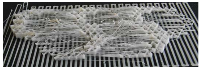
(a) Printed support (with thin strings)
