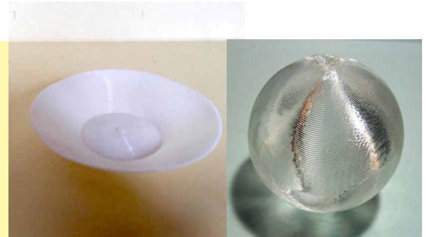
Objects with low-angle overhang (shallow plate and empty sphere)
